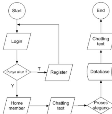
Fig. 4. Message Extraction Process Flowchart
